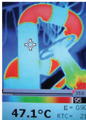
Thermal imaging shows the surface temperature of uninsulated piping (left) reduced by about half with 6 mm of Pyrogel® 6350 aerogel insulation (center). Photo at right shows fully insulated section of piping with elbows.
